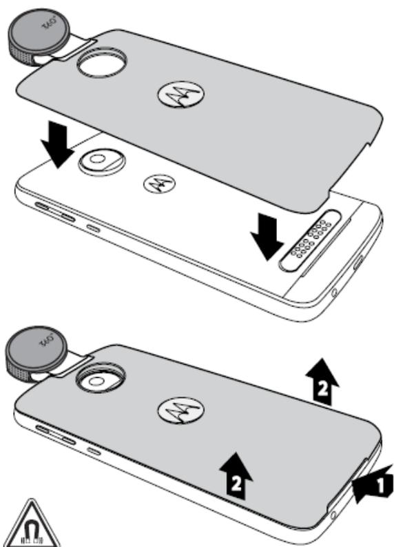
To remove the 360 Camera, lift up from the bottom.
